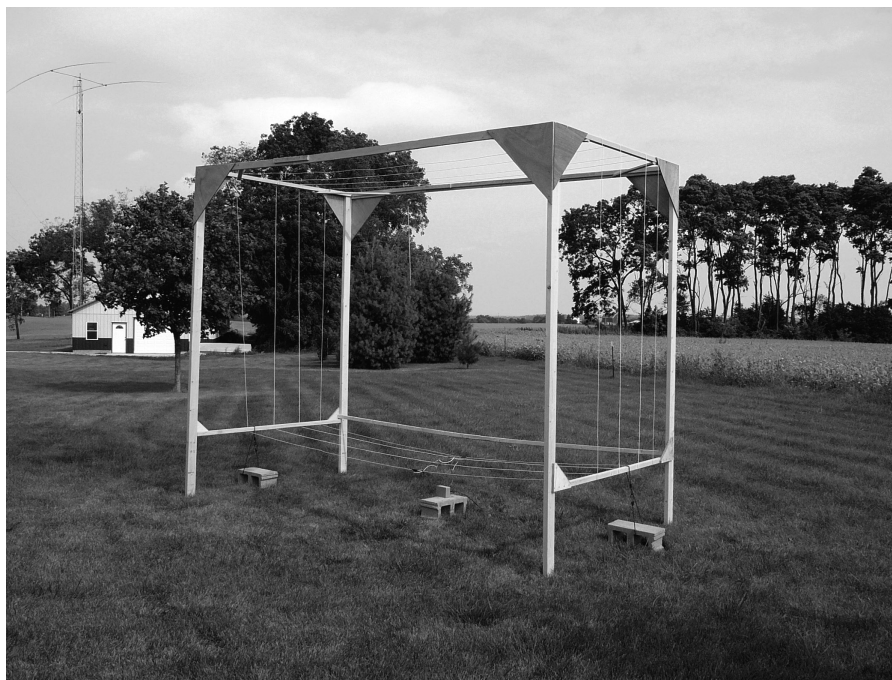
Figure 5 — Test setup used to evaluate several 8 × 12 multi-loop configurations. [Gary Breed, K9AY, photo]
